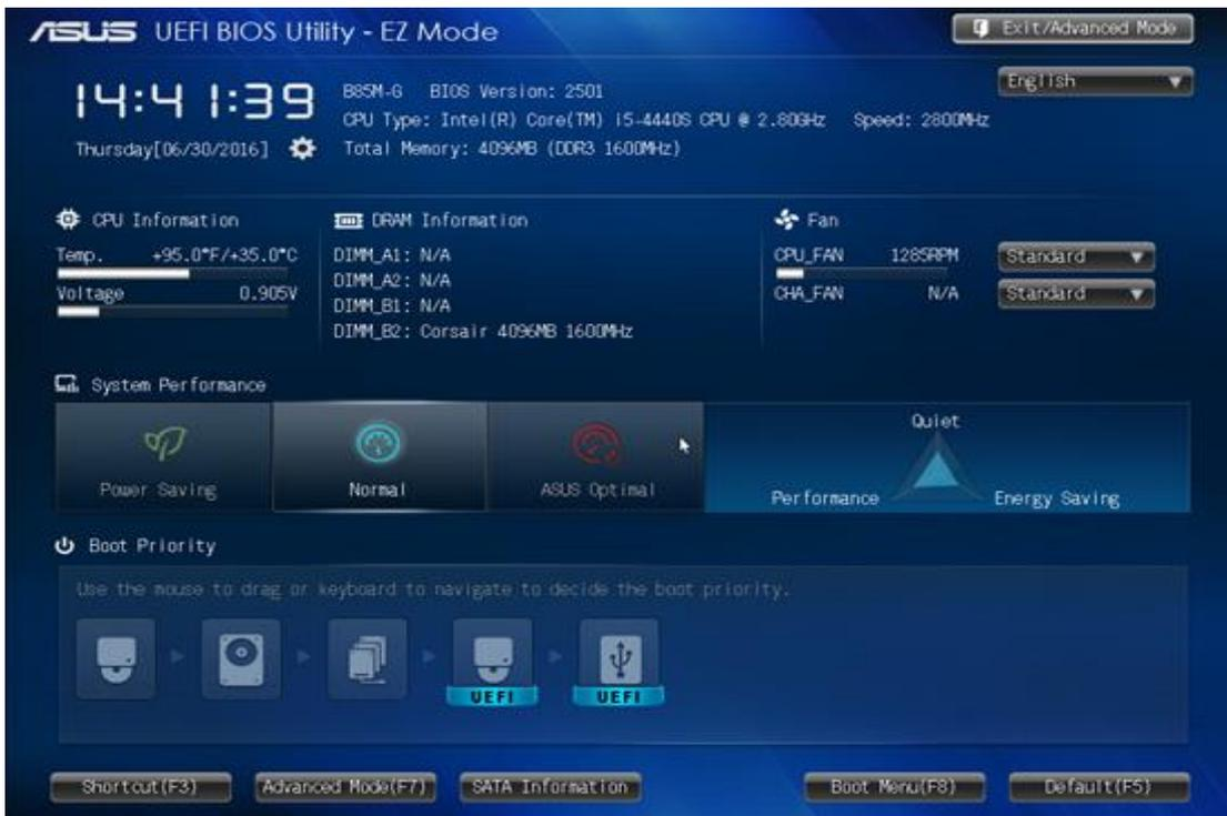
4. Click on **Advanced Mode** button or press <F7> function key to enter **Advanced Mode**. **Advanced Mode** screen is displayed as shown below:
